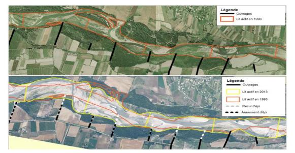
❑ Near the industrial area of Saint Maurice at Manosque, the cost of setting back 400m of dikes was 500k€ compared to 900k€ to strengthen the existing dikes close to the river (2016)
