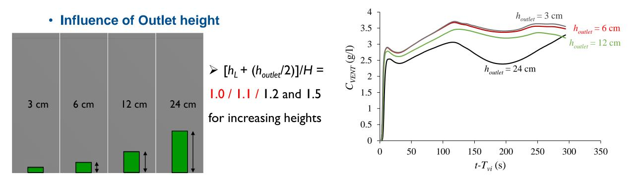
The height of the entrance of the outlet should be chosen in a way that the height of aspiration encloses the turbidity current body.
