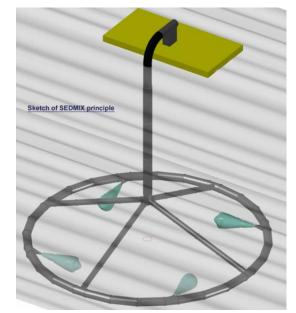
Outflow-jets in swirling flow, ascending effect On-demand operation Customized operation (space, time, flow rate) Potential energy or pumped supply Modular
