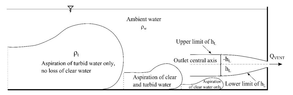
Where to place the outlet to increase the efficiency of venting?
