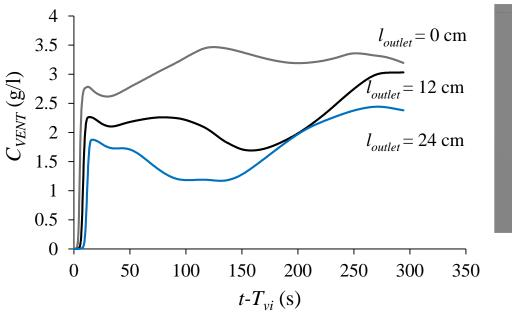
The outlet should be placed at the lowest level possible, minimizing the dead storage, for which the venting concentration remains the highest, the longest.
