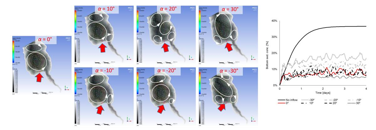
Outflow-jets have major influence in deep reservoir hydrodynamics and turbulence levels. Adequate jet orientation can significantly reduce sediment deposition
